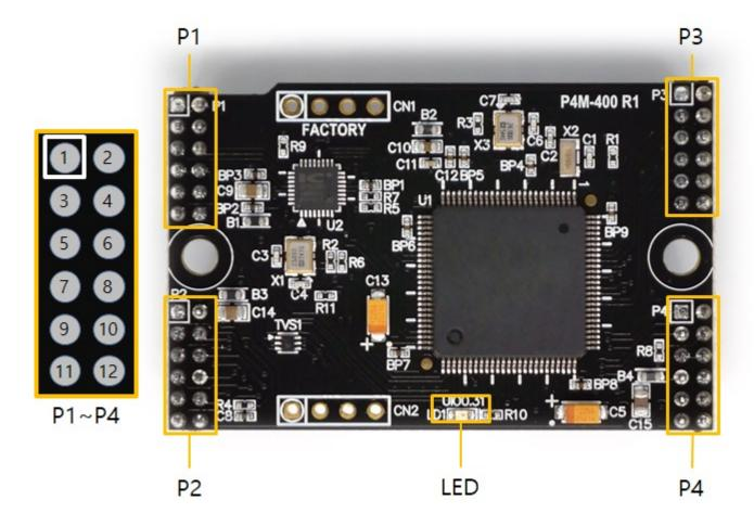
The P4M-400 interfaces with four 6 x 2-pin headers (P1 to P4). Space of each pin is 2 mm.
