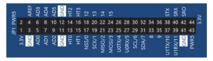
X JP1, JP2 and JP3 are designed to connect expansion boards for PHPoC boards.
