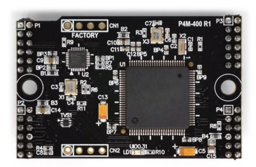
The P4M-400 is a module type of PHPoC product. Since PHPoC function is provided in module form, it is possible to implement the board suitable for user application.
