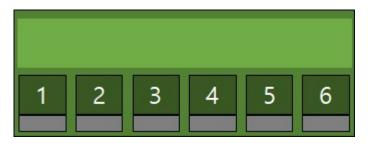
The type of serial port of P5H-152 can be selected to either RS485 or RS422. This port is a 6-pole terminal block and is mapped to UART0 for programming.
