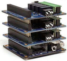
Smart Expansion Boards communicate with PHPoC Black/Blue as master and slave way through a smart expansion port. They can be stacked and recognized by each slave ID number among 14 different ID numbers which you can set by a dip switch. Two different types of terminal blocks are supported according to the direction of the terminal screw. S-type is convenient to screw from side when it is stacked. T-type is for you to screw from top.
