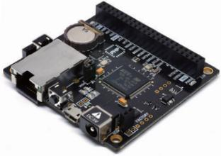
It is a wired LAN programmable board embedded with a PHPoC interpreter. It supports various interfaces to connect with sensors and equipment, and you can control your equipment from a remote site via web browser. Also, you can stack expansion boards to implement additional functions.
