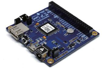
It is a wireless LAN programmable board embedded with a PHPoC interpreter. It supports various interfaces to connect with sensors and equipment and USB wireless LAN adapter is provided for network connectivity. Also, you can stack expansion boards to implement additional functions.
