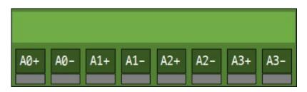
4 analog input ports are an 8-pole (3.5mm pitch) terminal block. Each port is mapped 0 to 3 channel of ADC device(ADC0/1/2) for programming. You must the input type of the each port. The input type will be voltage(DC 0  $\sim$  5V) when you output LOW to each input type select pin. On the other hand, the input type will be currentcurrent (0  $\sim$  20mA) when you output HIGH to the pin.
